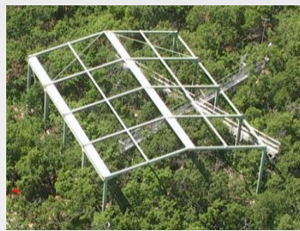
Figure 1: Dynamic rainfall exclusion system (~30% of annual precipitation) implemented in May 2012 at O 3 HP (Oak Observatory at the Observatory of Haute Provence, Saint-Michel-l'Observatoire).
